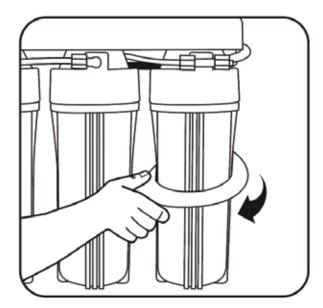
To open the bowls, use the housing spanner and turn clockwise.
