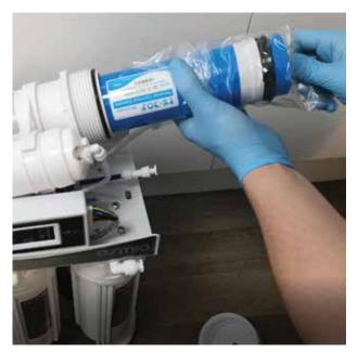
Insert the membrane into the membrane housing. Ensure it goes into the socket at the other end of the housing inside it and the membrane is flush with the top of the housing.
