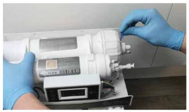
Insert the collet clip back into the push fitting
