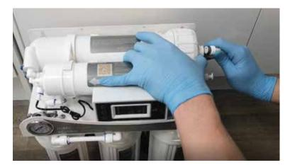
Insert the push fitting back into the membrane housing
