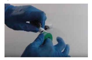
3) Then using your spanner, screw the ball valve into the feed in valve and tighten it with your spanner.
