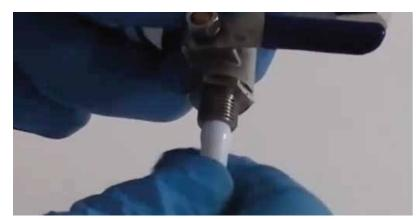
Push the tubing ontop the stem of the ball valve. Ensure it has been pushed all the way over the little ridge.
