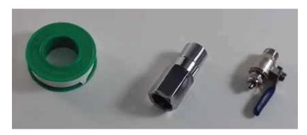
The feed in valve has 1/2" male and 1/2" female and a tee off. PTFE with 7 wraps the male end of the feed in valve and the male end of the blue lever ball valve.
