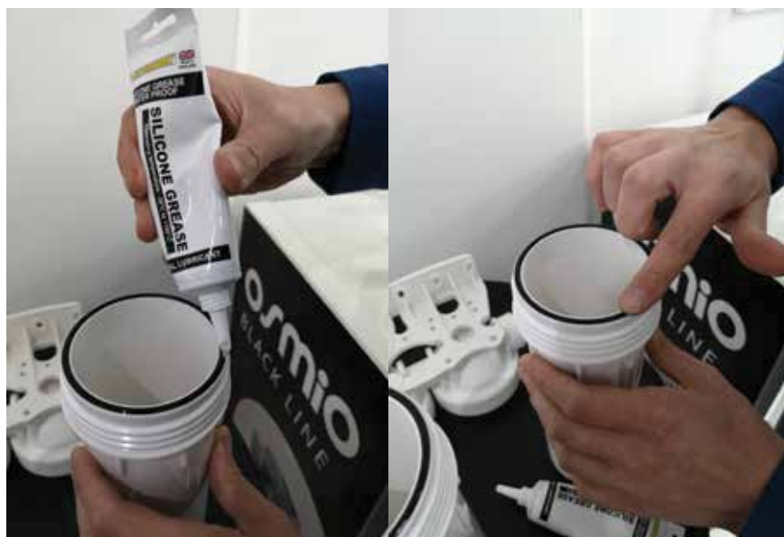
FIG4: GREASING THE O RINGS
