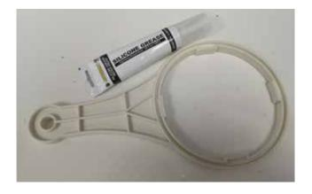
Leave a tube of silicone grease and the spanner next to the filter system. You will need it later!
