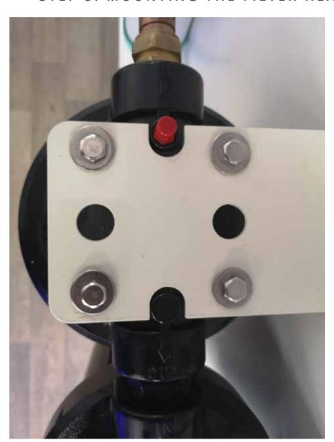
Use the screws provided with you filter housing to mount the bracket to the head of the filter unit. The screws are self-tapping and will thread themselves into the sockets of the housing head. Use a spanner or socket spanner for this.
